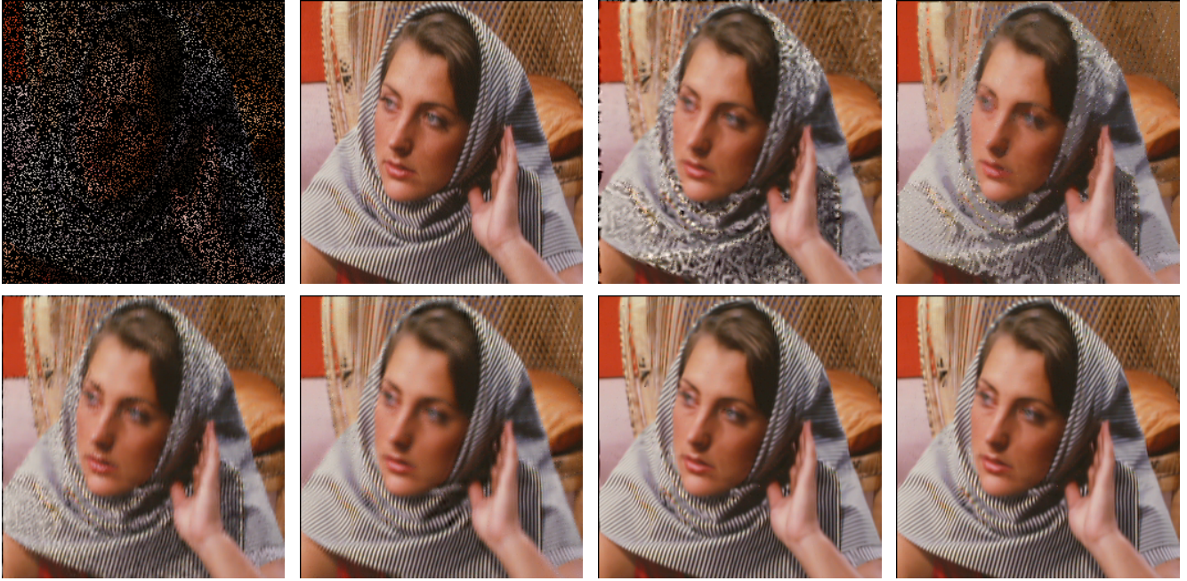
Figure 5: Visual quality comparison of image restoration from partial random samples for color image Barbara . From left to right and top to bottom: the degraded image with only 20% random samples available, original image, the recovered images by SKR [6] (PSNR=21.92dB; FSIM=0.8607), NLTV [35] (PSNR= 23.46dB; FSIM=0.8372), BPFA [48] (PSNR=25.70dB; FSIM=0.8926), HSR [10] (PSNR=28.83dB; FSIM=0.9273), SAIST [5] (PSNR=29.68dB; FSIM =0.9485) and the proposed GSR (PSNR=31.32dB; FSIM=0.9598).
