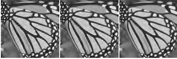
Fig. 2: Comparison of different methods at 0.25 bpp. Left: J2K (PSNR=23.18 dB, SSIM=0.7699); Middle: CADU (PSNR=23.24 dB, SSIM=0.7748); Right: WIDIC (PSNR=23.88 dB, SSIM=0.8130).
