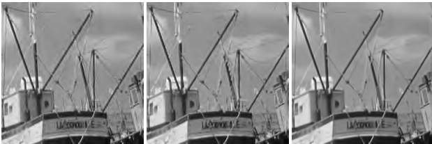
Fig. 5: Comparison of different methods at 0.35 bpp. Note the superior visual quality of the WIDIC method even though it has a lower PSNR. Left: J2K (PSNR=28.80 dB, SSIM=0.7906); Middle: CADU (PSNR=27.62 dB, SSIM=0.7847); Right: WIDIC (PSNR=28.37 dB, SSIM=0.7961).
