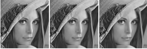
Fig. 3: Comparison of different methods at 0.25 bpp. Left: J2K (PSNR=29.82 dB, SSIM=0.8297); Middle: CADU (PSNR=29.83 dB, SSIM=0.8250); Right: WIDIC (PSNR=30.17 dB, SSIM=0.8340).
