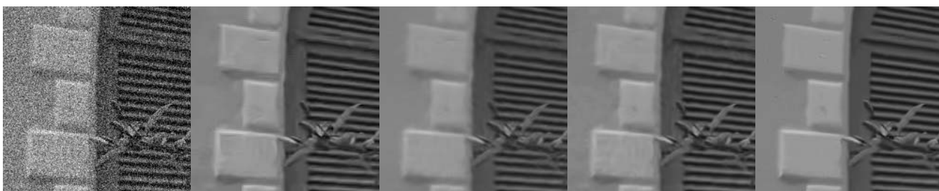
Figure 6. Perceptual comparison for Window . From left to right: (a) Noisy image ( \sigma_n = 30 ); (b) BM3D (PSNR = 30.49dB); (c) LPG-PCA (PSNR = 29.76); (d) CSR (PSNR = 30.63dB); (e) Proposed (PSNR = 30.92dB).
