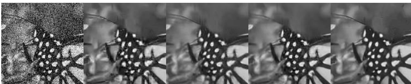
Figure 7. Perceptual comparison for Monarch . From left to right: (a) Noisy image ( \sigma_n = 40 ); (b) BM3D (PSNR = 25.77dB); (c) LPG-PCA (PSNR = 26.14); (d) CSR (PSNR = 26.81dB); (e) Proposed (PSNR = 27.17dB).
